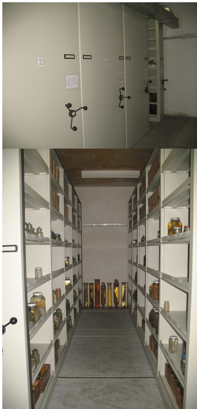
Figure 3. Mobile shelving system used to store jar specimens in the Ichthyological Collection of the Museu Nacional, Universidade Federal do Rio de Janeiro.
